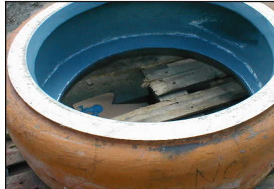
ARC BX2* and ARC MX1 with a top coat of ARC 855
