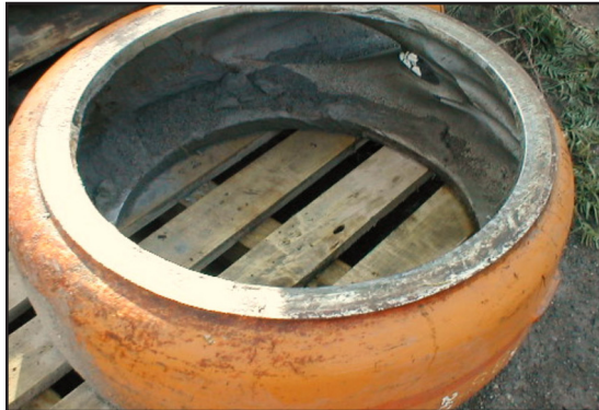
Worn pump casing
